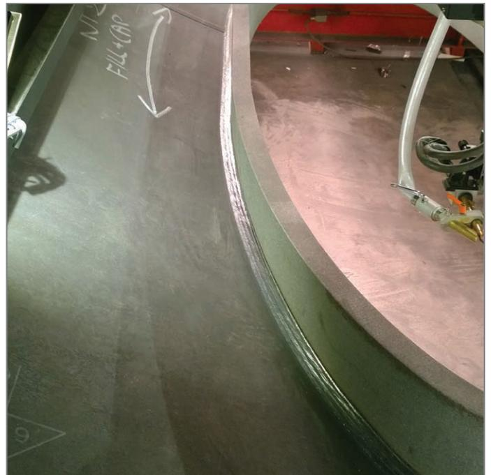
MCM door frame scanning, oxy cutting/beveling and SAW welding / One-man operation.
