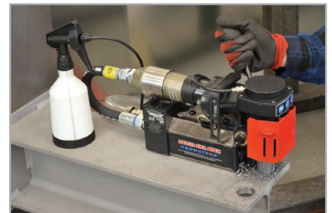
Through spindle cooling system
