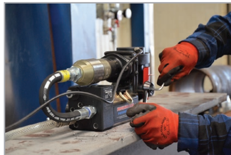
Feed lever can be fixed from either side
